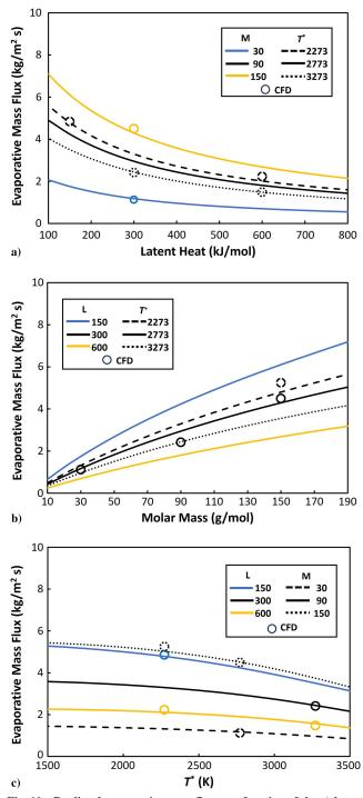
Fig. 10 Predicted evaporative mass flux as a function of the a) latent heat of evaporation, b) molar mass, and c)  $T^*$ .
