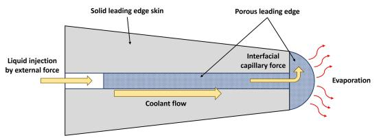
Fig. 1 Schematic of transpiration-cooling TPS utilizing liquid coolant and porous leading edge.
