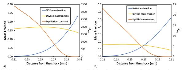
Fig. 17 Mass fractions and equilibrium constants for O and a) SiO<sub>2</sub> and b) BaO as a function of distance away from the surface at the stagnation point.
