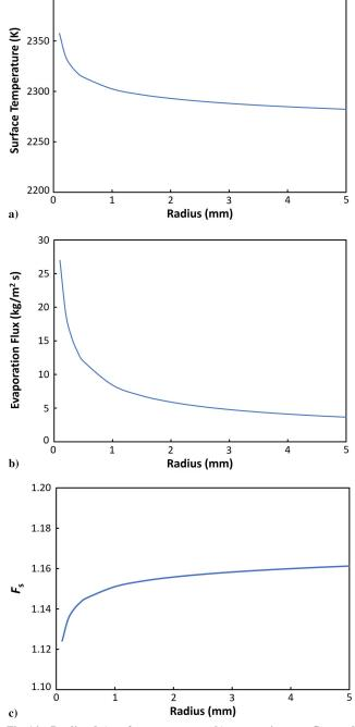
Fig. 14 Predicted a) surface temperature, b) evaporative mass flux, and c)  $F_s$  as a function of leading edge radius for edge radius.
