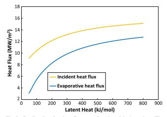
Fig. 8 Predicted surface heat fluxes as a function of the latent heat. The molar mass and  $T^*$  of the material are 90 g/mol and 2773 K.
