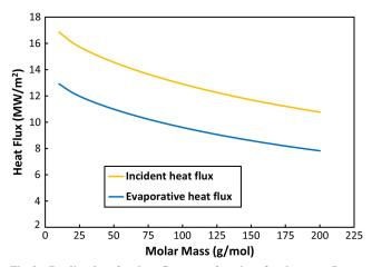
Fig. 9 Predicted surface heat fluxes as a function of molar mass. Latent heat and  $T^*$  of the material are 300 kJ/mol and 2773 K.
