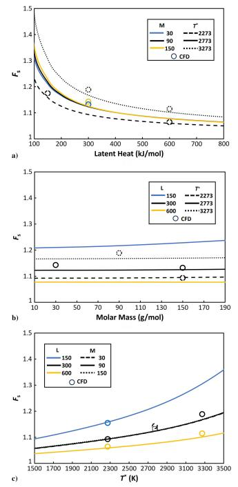
Fig. 11 Predicted  $F_s$  as a function of the a) latent heat of evaporation, b) molar mass, and c)  $T^*$ .
