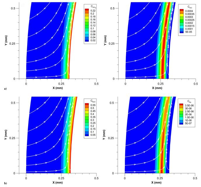
Fig. 16 Mass fraction color contours of a) SiO<sub>2</sub> and b) BaO and their dissociates near the leading edge, with streamlines shown in white lines.
