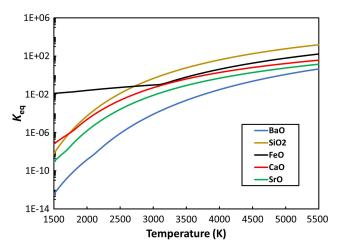
Fig. 18 Equilibrium constants of typical oxides, including BaO and  $SiO_2$ , as a function of temperature.
